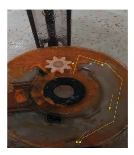
27. The Defendant denies that the contested embodiment implements the feature. It points out that the groove around the through hole has no connection to the juice outlet and
